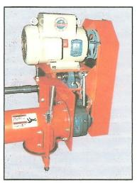
The exit auger closing hatch is easy to operate and requires only minimum opening clearance. This provides more room beneath the unloader for conveyors and auxiliary equipment.
